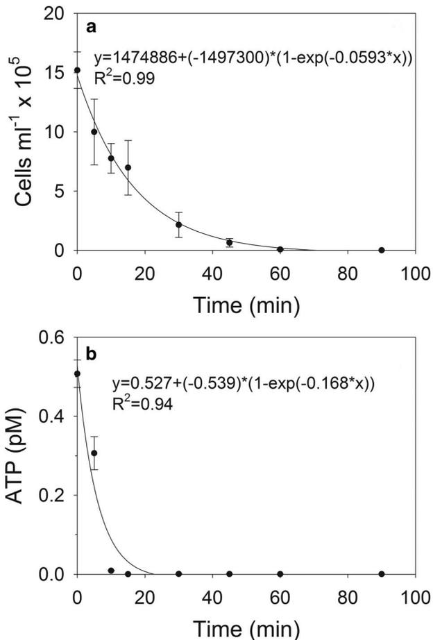
**Fig. 6. a.** Pond water cell, and **b.** adenosine triphosphate (ATP) concentrations in the tank at a flow rate of  $761 \text{ min}^{-1}$  with the samples passing through both filter systems and both UV lamps. Each time point represents the mean and standard error (s.e.) ( $n = 3$ ). Cell concentrations and ATP levels were below levels of detection after 60 min and 15 min, respectively.
