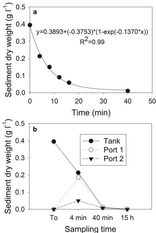
**Fig. 5. a.** Sediment concentration in the tank over time, and **b.** in the tank and ports 1 and 2 at specific times up to 15 hours. Water was recirculated through the tank during this experiment, passing only through the  $2 \mu\text{m}$  filter, at a flow rate of  $951 \text{ min}^{-1}$ .
