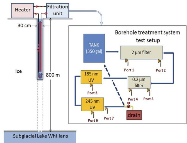
**Fig. 2.** Schematic (left panel, not to scale) showing the flow directions for the field operation of the Whillans Ice Stream Subglacial Access Research Drilling (WISSARD) water treatment system. The filtration and UV-treatment unit will be placed in-line between the borehole water return line and the heater modules. The enlarged inset (right panel) shows the treatment system components as set up for the laboratory tests. See text for details.
