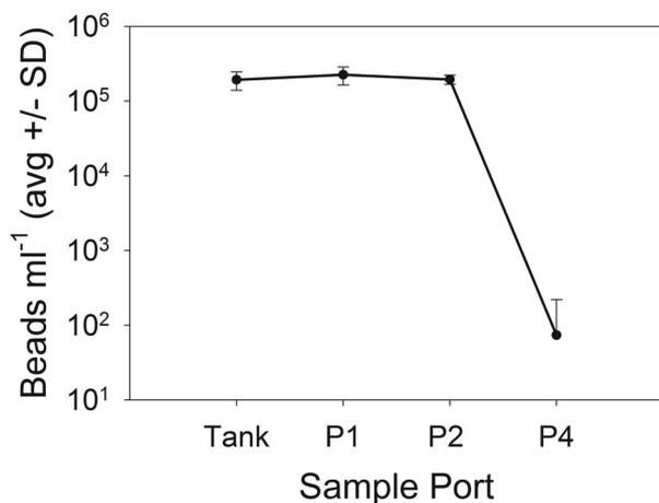
**Fig. 4.** Fluorescent beads counted from the tank and selected sample ports after filtering 11131 through the system. The flow rate was  $\sim 941 \text{ min}^{-1}$ . Error bars = standard deviation (SD) ( $n = 4$ ).
